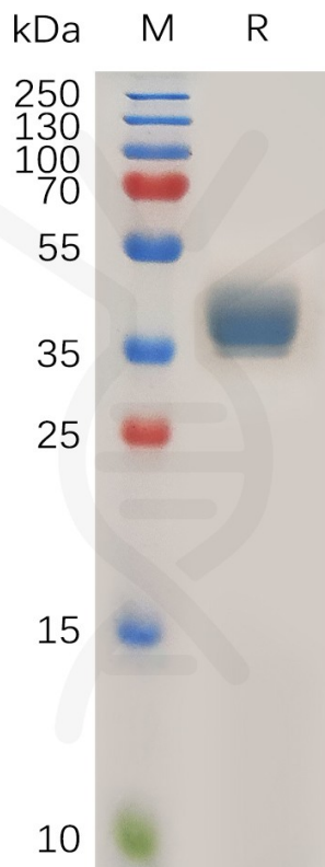
Figure 1. Human CCR1 Protein, hFc Tag on SDS-PAGE under reducing condition.
