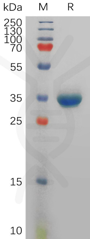
Figure 1. Human PYY Protein, hFc Tag on SDS-PAGE under reducing condition.
