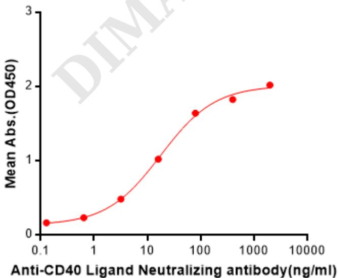
Figure 1. ELISA plate pre-coated by 2  $\mu$ g/ml (100  $\mu$ L/well) Human CD40 Ligand Protein, hFc Tag (PME100192) can bind Anti-CD40 Ligand (ruplizumab biosimilar) mAb (BME100042) in a linear range of 0.64-400 ng/ml. In order to specifically detect BME100042, mouse anti-human Fab-specific antibody was used as detection antibody.
