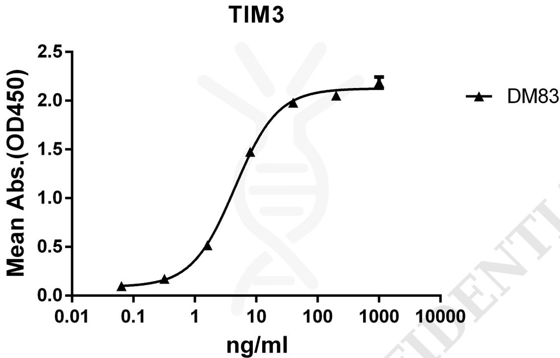
Figure 1. ELISA plate pre-coated by 2  $\mu\text{g/ml}$  (100  $\mu\text{l/well}$ ) Human TIM3 protein, mFc-His tagged protein PME100030 can bind Rabbit anti-TIM3 monoclonal antibody ( clone: DM83) in a linear range of 0.32-40 ng/ml.
