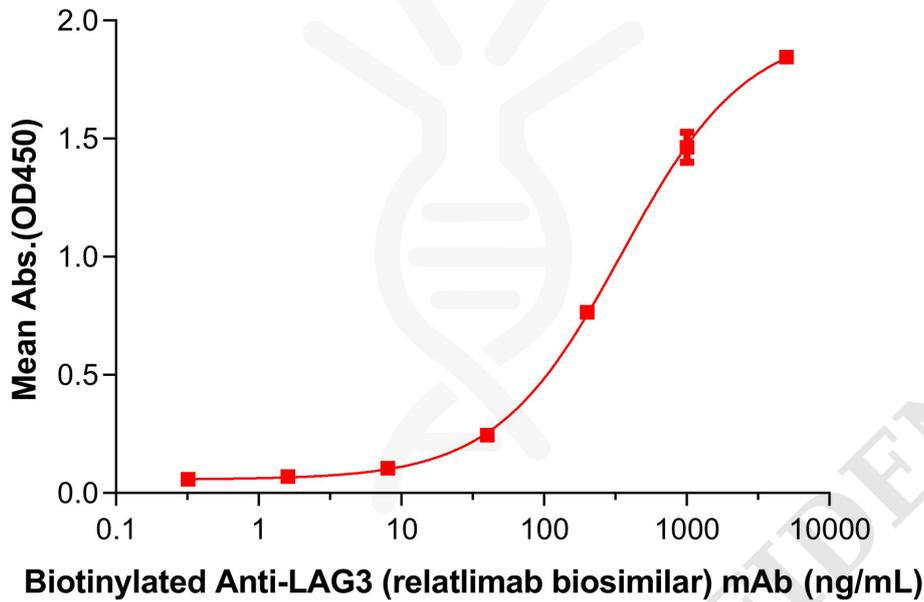
Figure 1. ELISA plate pre-coated by 2  $\mu$ g/mL (100  $\mu$ L/well) Human LAG3 Protein, His Tag (PME100512) can bind Biotinylated Anti-LAG3 (relatlimab biosimilar) mAb (BME100062B) in a linear range of 200-1000 ng/mL.
