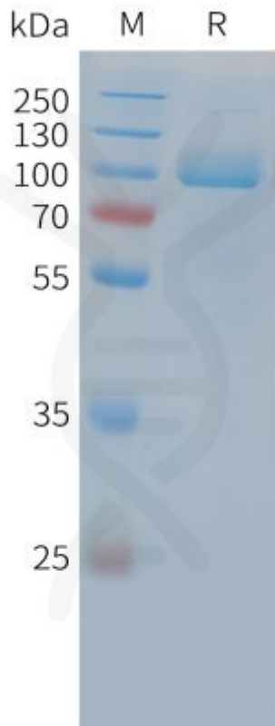
Figure 1. Cynomolgus PSMA Protein, His Tag on SDS-PAGE under reducing condition.
