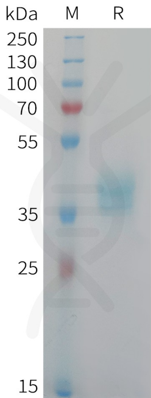
Figure 1. Human CADM3 Protein, His Tag on SDS-PAGE under reducing condition.
