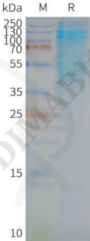
Figure2. Human CD37-Nanodisc, Flag Tag on SDS-PAGE
