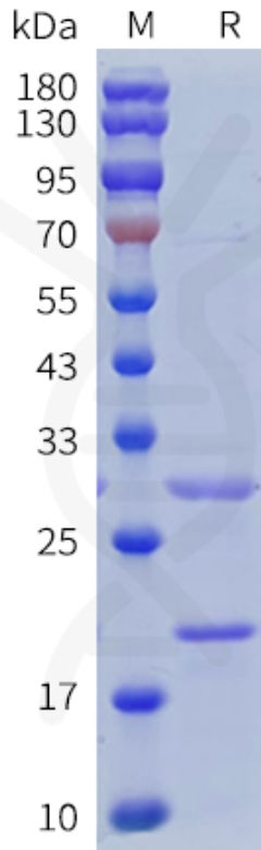
Figure 1. Human CLDN1 cell-free-Nanodisc,C-Single Strep&His Tag on SDS-PAGE.
