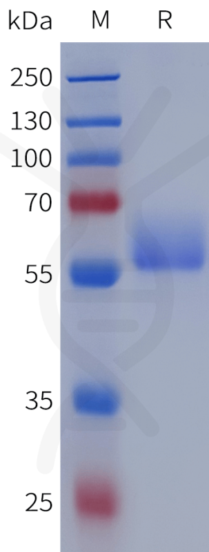
Figure 1. Human EGFR(446-621) Protein, hFc Tag on SDS-PAGE under reducing condition.
