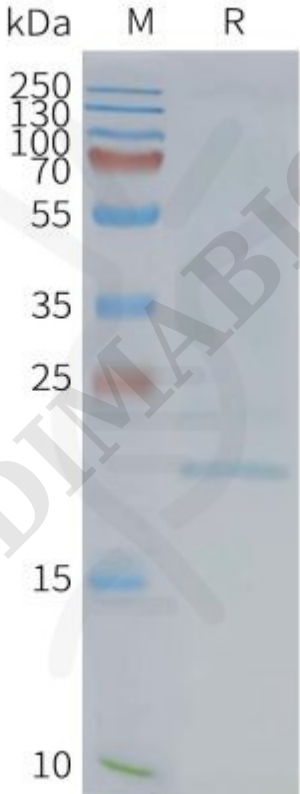
Figure2. Human EMP2-Nanodisc, Flag Tag on SDS-PAGE
