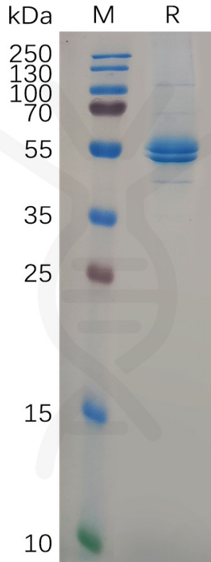
Figure 1. Human IL11 Protein, hFc Tag on SDS-PAGE under reducing condition.
