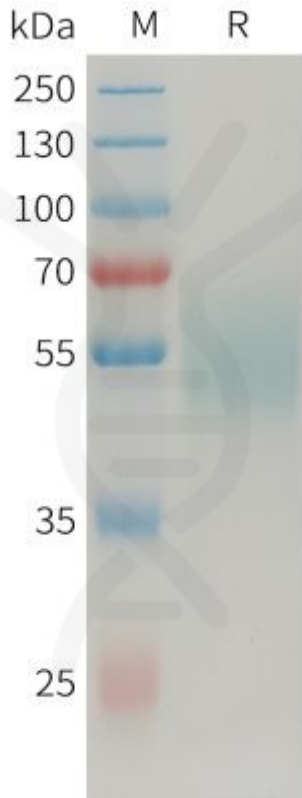
Figure 1. Human MICA \alpha 3 Protein, mFc Tag on SDS-PAGE under reducing condition.
