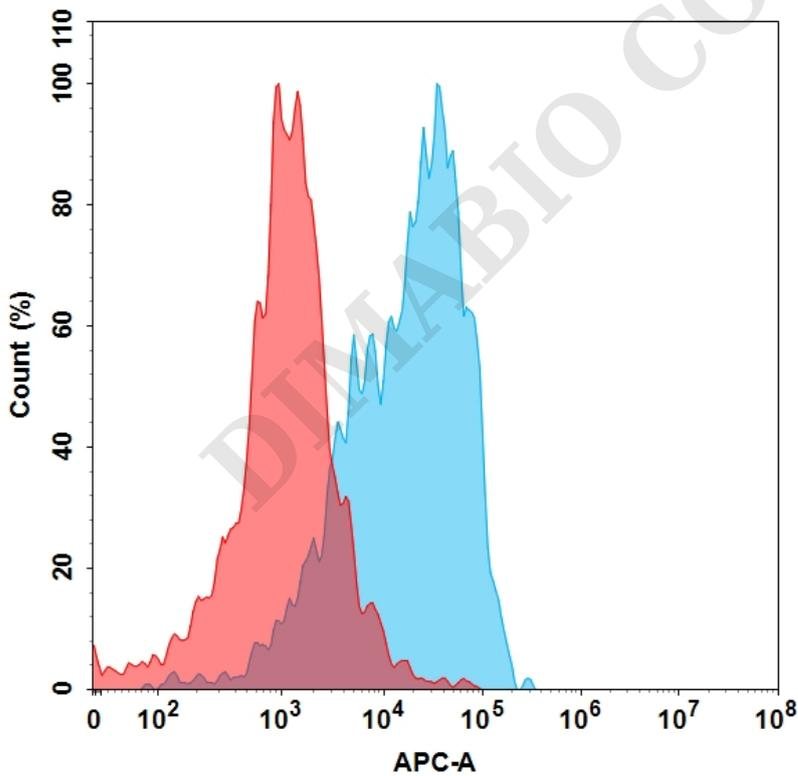
Figure 3. Flow cytometry analysis with 15  $\mu\text{g/mL}$  Human MICB Protein, His Tag (PME100516) on HEK293 cells transfected with Human NKG2D protein and Human DAP10 protein (Blue histogram) or HEK293 transfected with irrelevant protein (Red histogram).
