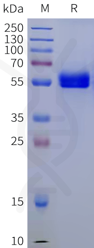
Figure 1. Mouse CD8A Protein, hFc Tag on SDS-PAGE under reducing condition.
