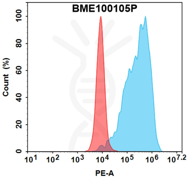
Figure 1. Flow cytometry analysis with 100  $\mu$ l/test (1:400) PE-conjugated Anti-CCN2(pamrevlumab biosimilar) mAb (BME100105P) on HEK293 cells transfected with Human CCN2 protein (Blue histogram) or HEK293 transfected with irrelevant protein (Red histogram).
